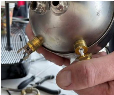
20. Use a 17mm wrench to loosen the klixons, then remove
