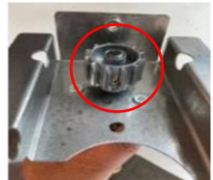
6. Using the long Schaerer screwdriver, remove the two set screws from the gear and slide it off the shaft
