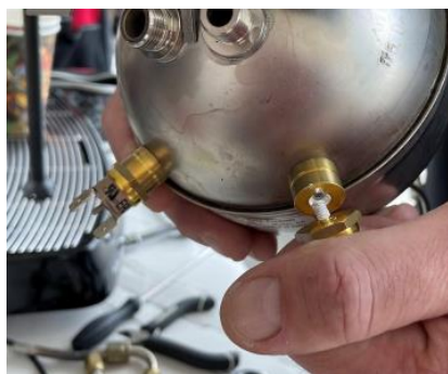
16. Do not use tools to tighten the klixons, only hand tighten
