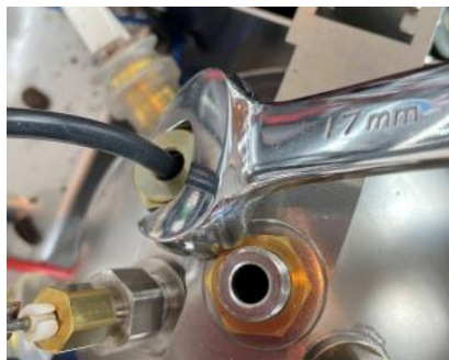
14. Using a 17mm wrench, remove the temp sensor and inlet pipe
