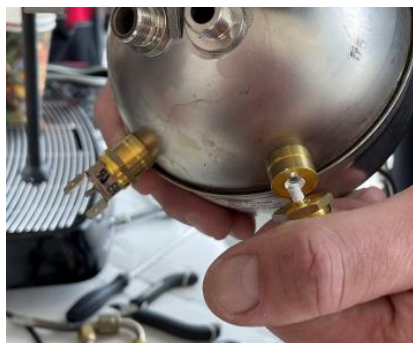
13. Apply a very thin layer of thermal paste to the klixon support
