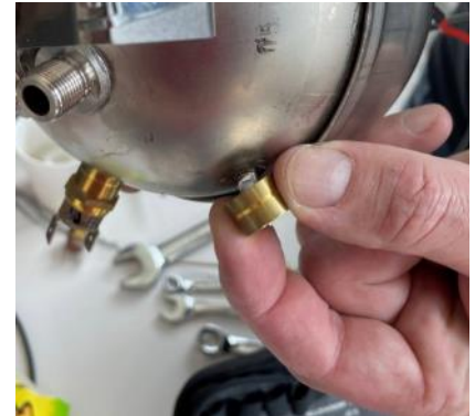
12. Clean dried thermal paste from used klixon support
