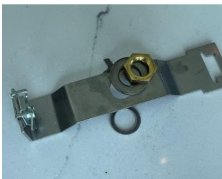
23. Transfer Fiber Gasket, Bracket, washer and nut to new boiler
