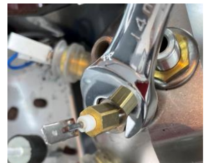
15. Using a 14mm wrench, remove the level probe (note: do not lose the washer)
