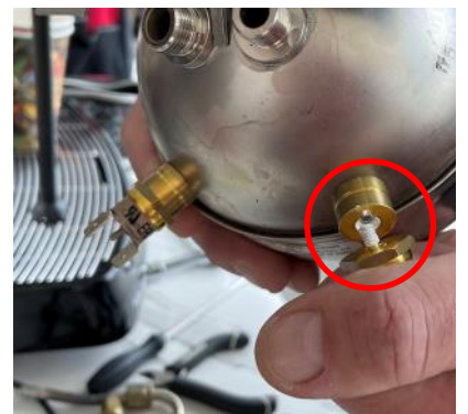
25. Apply a very thin layer of thermal paste to the klixon support
