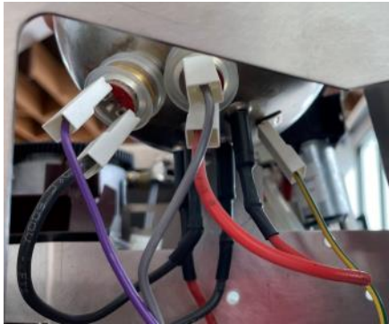
17. Disconnect the lower klixon and element wires and ground wire.
