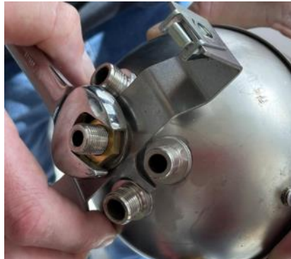
11. Use a 17mm wrench to remove the boiler support bracket. Set
