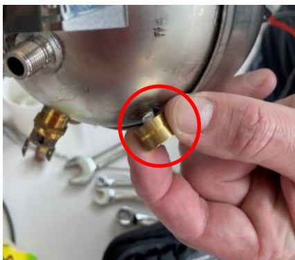
24. Clean dried thermal paste from used klixon support
