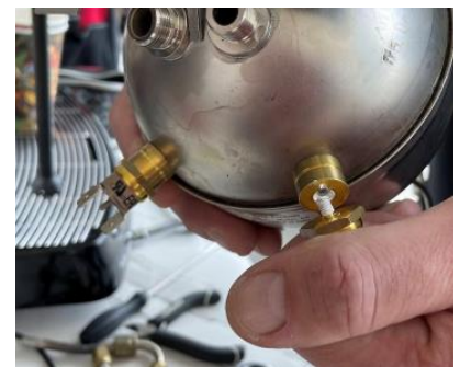
15. Apply a thin layer of thermal paste to top of the support and
