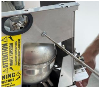
16. Remove the fastening screw for the boiler support bracket
